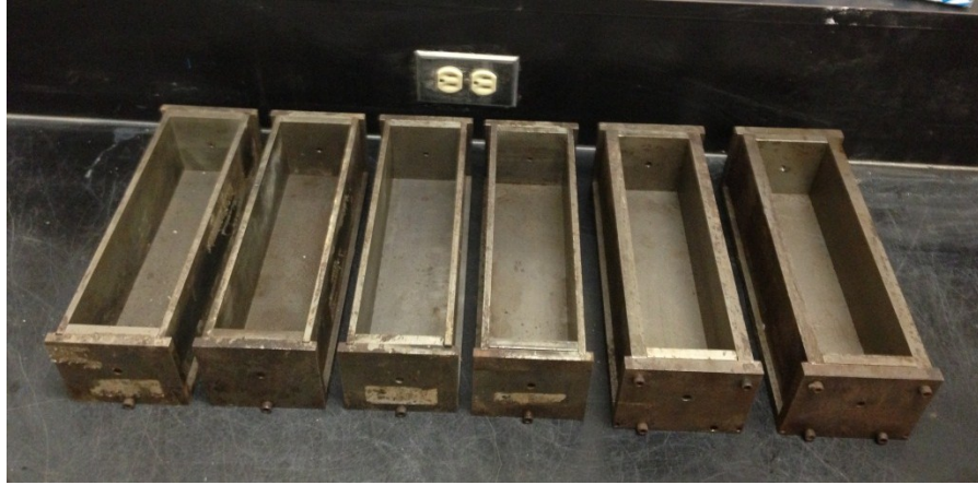
Figure 4.11: 3 x 3 x 11.25 in. concrete prism molds
