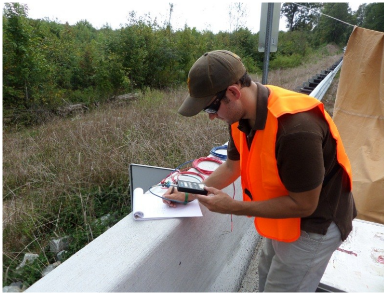
Figure 3.36: VWSG readings being collected with Geokon GK-404 readout system
