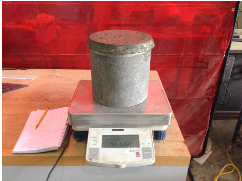
Figure 4.10: Concrete unit weight test
