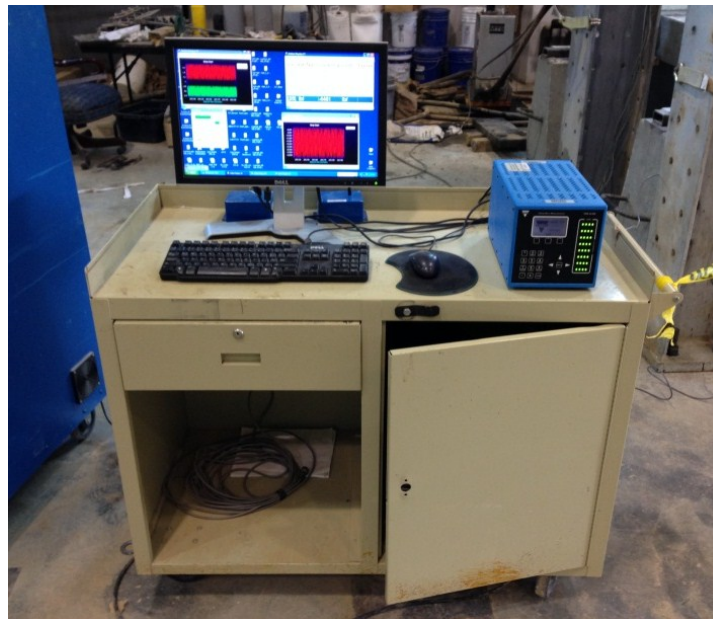
Figure 3.19: Vishay Micro-Measurements System 7000 and Strain Smart data acquisition system
