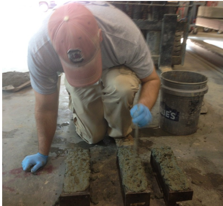
Figure 4.12: Casting of specimens
