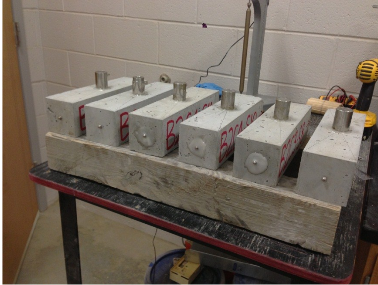
Figure 4.16: Batch 2 specimens with AE sensors attached
