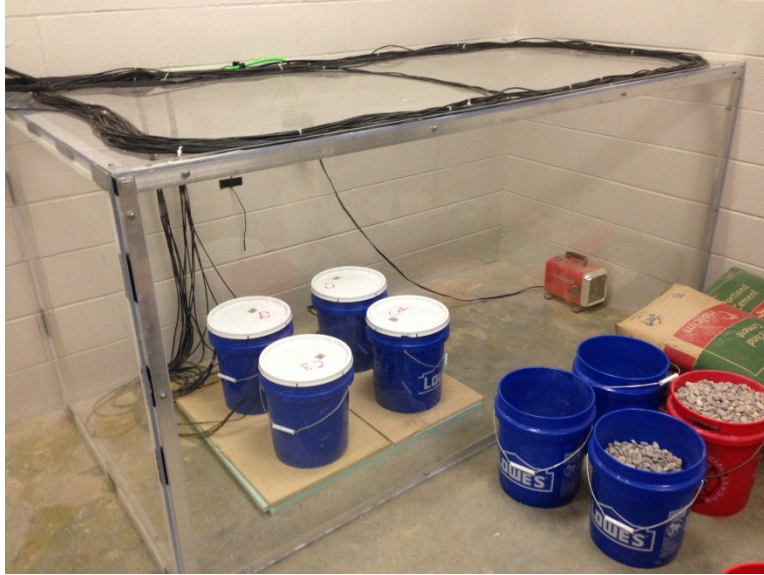
Figure 4.1: Temperature controlled testing chamber
