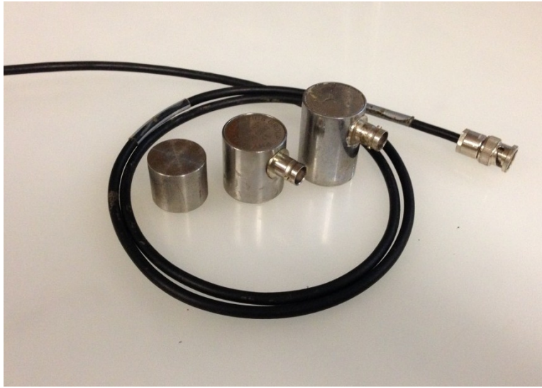
Figure 4.20: R6i (right) and WDi (middle) sensors, sensor cable, and counter weight (left)
