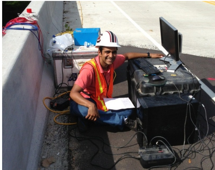
Figure 3.39: On-site 7000 System and Strain Smart software data acquisition system setup
