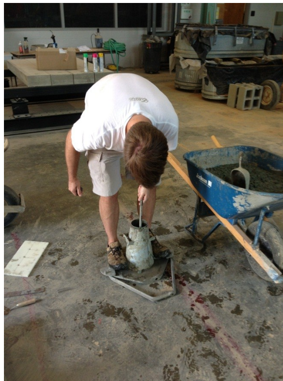
Figure 4.8: Slump test being performed
