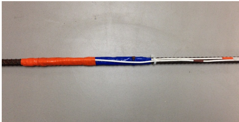
Figure 3.17: ERSG attached to No. 4 sister bar, fully waterproofed
