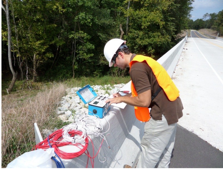
Figure 3.37: ERSG readings being collected with Vishay P3 strain indicator
